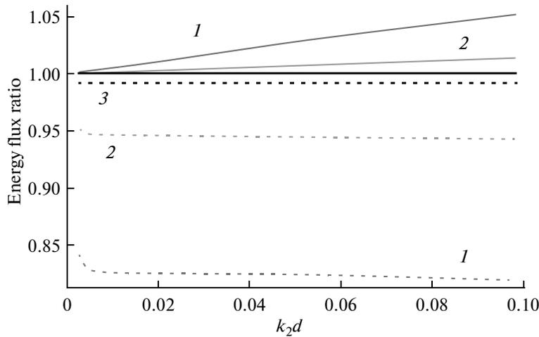
**Fig. 6.** Frequency dependence of radiation by a source with finite dimensions. Power fluxes  $E^+$  (solid lines) and  $E^-$  (dashed lines) generated by  $M$  sources with relative size of  $a/d = 0.9$  (1),  $0.6$  (2), and  $0.3$  (3) are normalized to the corresponding power fluxes from equivalent point sources.
