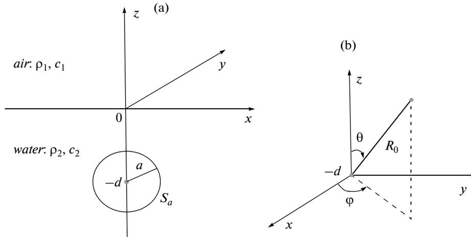
Fig. 1. Geometry of the problem (a) and local spherical coordinates (b).
