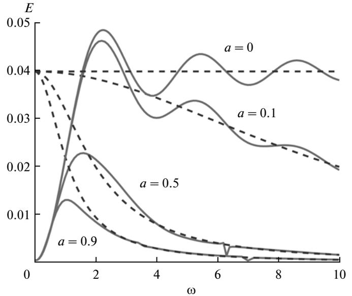
**Fig. 5.** Frequency dependence of total radiated power  $E$  of a point ( $a = 0$ ) and three spherical  $M$  sources (solid lines) and the power  $E_0$  radiated by these sources into a homogeneous space (dashed line).
