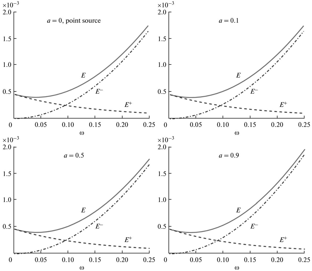
**Fig. 3.** Low-frequency distribution of the total radiated power  $E$  between energy fluxes  $E^+$  and  $E^-$  for point ( $a = 0$ ) and spherical  $M$  sources of different radius  $a$ .
