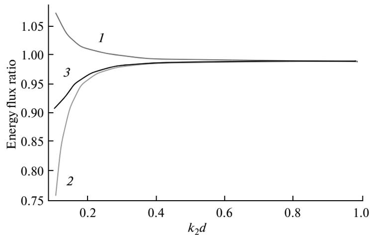
**Fig. 7.** Sound emission by a source with a small wave dimension at different distances to the water–air interface. The ratios of the power fluxes generated by an  $M$  source and by a point source that go to infinity in air (1) and water (2) and the ratio of the total radiated acoustic powers (3) are shown as functions of dimensionless depth  $k_2d$  of the sources. The radius of the  $M$  source is  $a = 0.1\kappa_2^{-1}$ .
