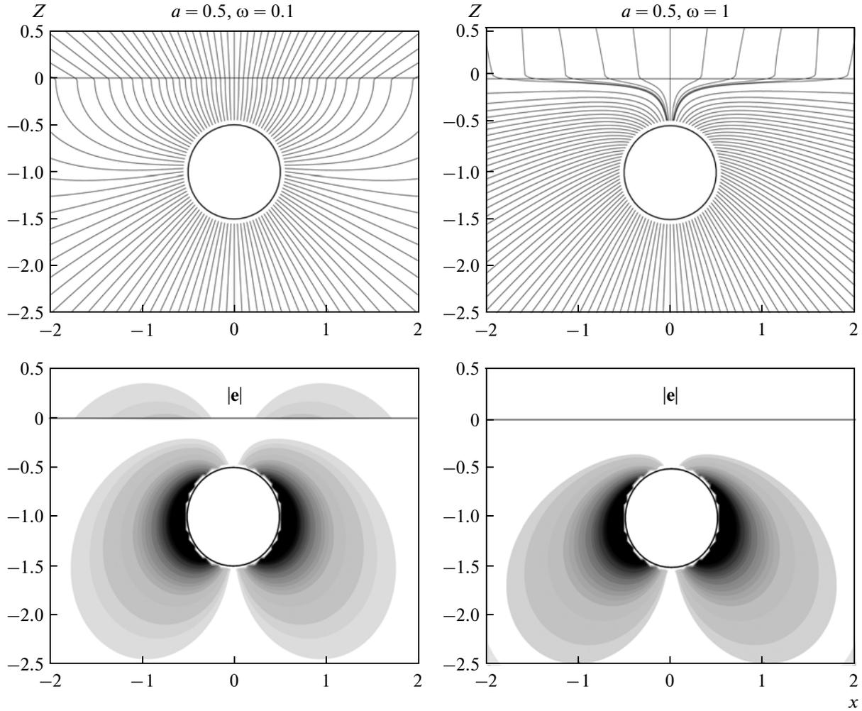
**Fig. 4.** Energy streamlines (top) and energy flux density  $|e(x, z)|$  (bottom) for an  $M$  source of radius  $a = 0.5$  and low ( $\omega = 0.1$ , left) and medium ( $\omega = 1$ , right) frequencies.
