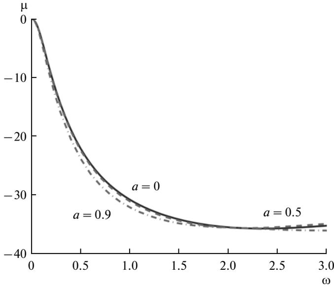
**Fig. 2.** Frequency dependences of transparency coefficient  $\mu$  illustrating the weak influence of the relative size of a spherical emitter on the given characteristic.
